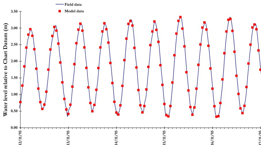
There is excellent agreement between the modelled and field data. Secondly, measured and modelled cumulative water volumes through cross section over a tidal cycle are compared. Volumes are considered as positive during the flood tide and negative during the ebb tide. The maximum cumulative volume during the tidal cycle defines the tidal prism. There are many factors that determine this volume at any one time i.e.:
