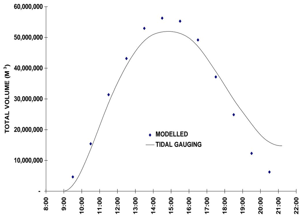
Many other comparisons between field measurements and modelled data were carried out which are not reported here for the sake of brevity but ensure that the model parameters were optimised. We are confident that for a wide range of freshwater inflows and tides, currents and water level within the Mahurangi estuary can be predicted.
